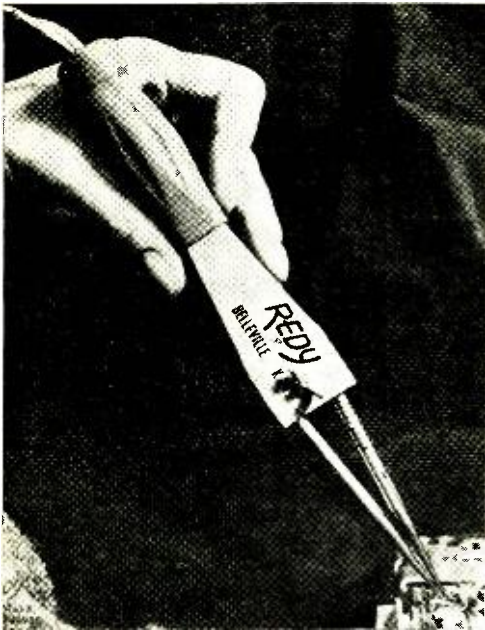
This is a tweezer-type electrode assembly that is commonly used with resistance soldering equipment.
