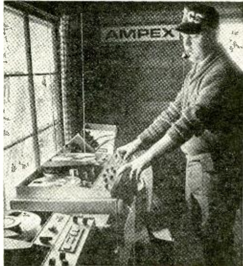
Jim Peterson, Technical Supervisor, Ampex Video Institute, makes last minute checks prior to taping skiing events by Interski teams. Unit on his belt is CB receiver; transceiver is between recorders.
