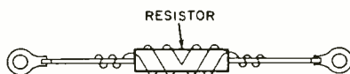
Fig. 2. Correct method of winding a noninductive shunt, winding from center to ends, is shown here.
