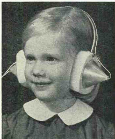
To make the headset comfortable, the funnel edge should be padded with foam rubber or plastic foam. Cement in place after making the necessary cutout. Headset is very light in weight.
