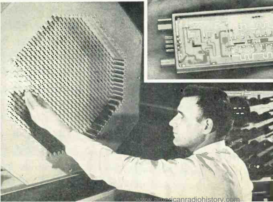
Solid-state microwave radar module (right) includes transmitter, receiver and antenna. Texas Instruments uses 604 modules to make airborne phased antenna radar array (below).
