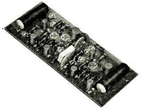
Fig. 12. The author's prototype of the straight preamplifier before installation of transistors.
