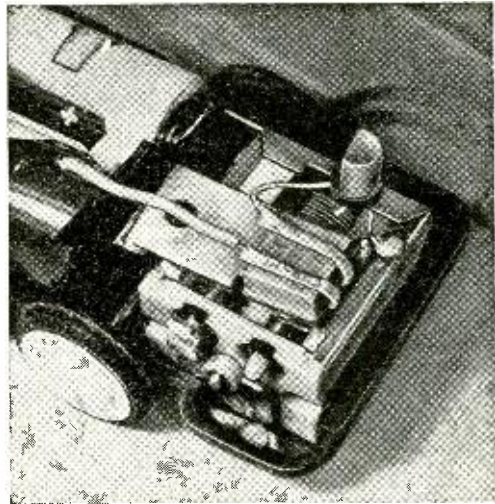
Plastic-encapsulated transistor saves space and gives neat appearance to station wagon installation.
