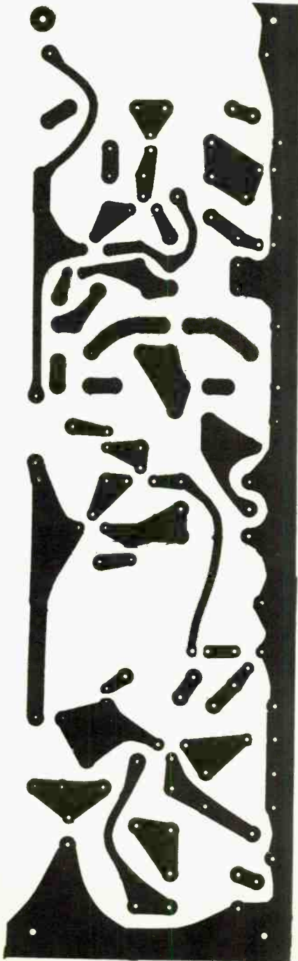
Fig. 6. Actual-size printed board for assembly of instrument preamplifier. The preamp can also be used independently with any instrument audio system.
