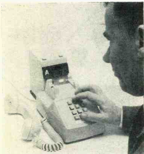
Bell Telephone Laboratories developed this experimental device to enable deaf people to use phone.
