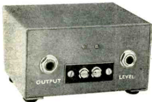
Rear view of COMPLY unit shows terminal strip for connection to external 9-volt power source. A screwdriver-adjusted pot is used for level setting.
