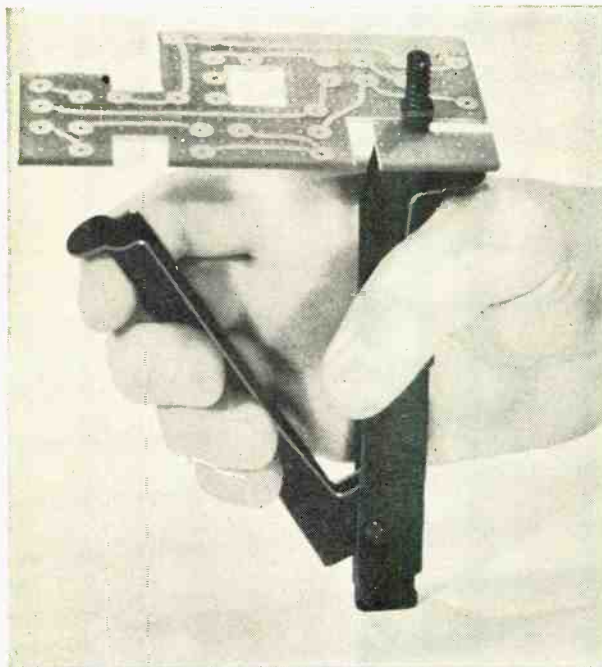
Fig. 1. A nibbling tool trims, notches, or cuts up to 18-gauge steel, 1/16" aluminum, and all types of plastic PC boards.
