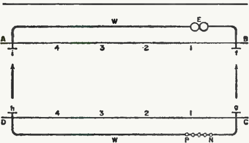
In diagram drawn by Samuel Morse, AB and CD represent opposite banks of a river; f, g, h, and i are copper plates (antenna); w indicates wires; and PN and E are batteries and headphones respectively.
