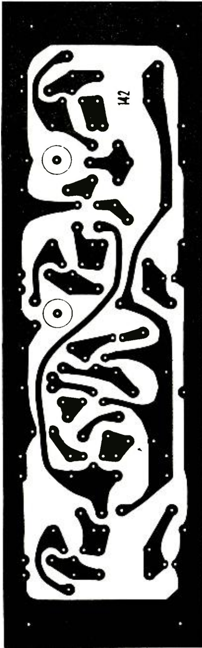
Fig. 2. Actual-size printed circuit board etching guide is shown at (A); dashed line in component layout guide (B) indicates insulated jumper wire.
