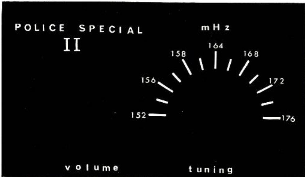
Fig. 4. Actual-size calibration guide can be copied or cut out and cemented directly on front panel.
