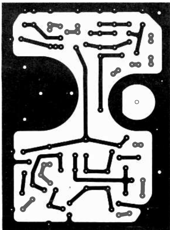
Fig. 2. "Same-size" outline of printed circuit board for readers who like to make their own. In drawing above, right, are notations on drilling of holes and making external connections to the printed circuit.
