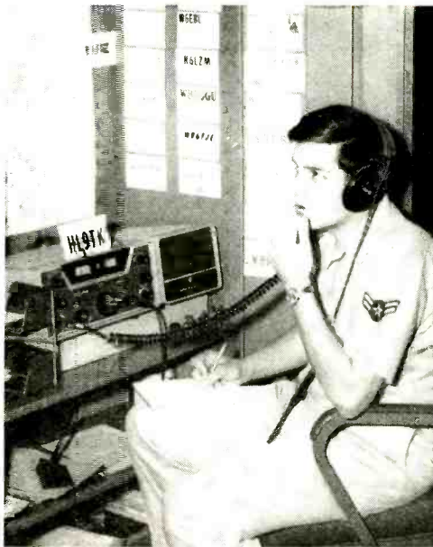
Airman Second Class John Ferrara initiated rescue operation at sea with his Hallicrafters SR-150 transceiver, running 100 watts PEP, and a Mosley V-3 Junior vertical whip antenna. (USAF Photo)
