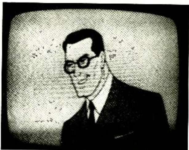
Home antenna installation brought in satisfactory picture quality from Channels 2, 6, and 9. A mast-mounted amplifier could eliminate most of the snow.
