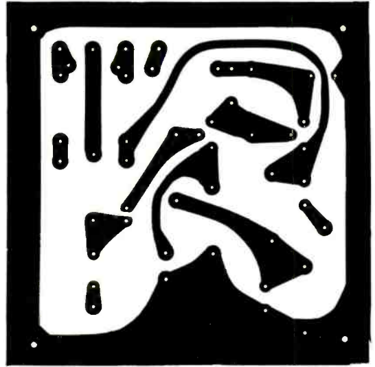
Fig. 5. Same-size layouts of the foil side of the two printed circuit boards are shown above. The fixed-gain preamplifier is to the left and the tone control board to the right. For stereo operation the builder requires 4 boards, two of each circuit.
