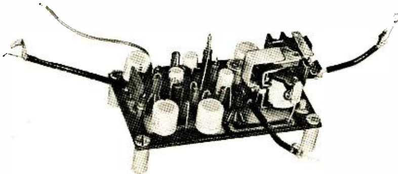
Fig. 5. Completed board assembly. Note use of shielded cable for input and output connections. Stand-offs are used to mount the board in the cabinet and to provide clearance. Components are stood on end.
