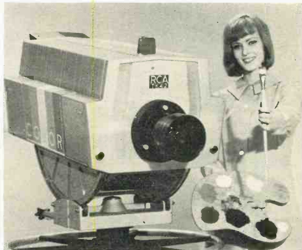
Latest in studio color cameras from RCA costs over $70,000, is fully transistorized, and has 4 camera tubes—1 for each primary color, 1 for luminance.
