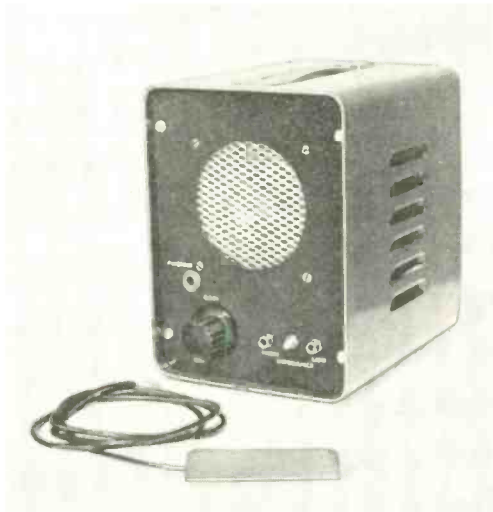
Both the Hydronics receiver and its speaker can be housed in the same cabinet, as shown here. For concentrated listening, a microphone jack can be used.
