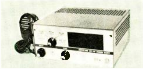
Five channels and 35 watts of radiated power are features of Hartman's "Hurricane" transceiver.
