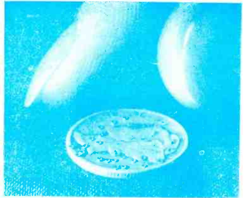
MICROMINIATURE CORES TO GUIDE SATURN —To get the most guidance information into the smallest possible space, IBM engineers designed microminiature cores for the Saturn IB launch vehicle's guidance computer. Some 545 cores fit on a dime.
