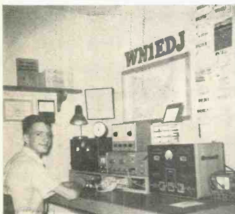
Gary Confrey, WN1EDJ, Killingworth, Conn., is shown here before the arrival of his General Class license. Gary's Hammarlund HQ-120 receiver, Lafayette "Starlite" transmitter, and 40-meter dipole antenna worked 23 states and Canada in 4½ months.
