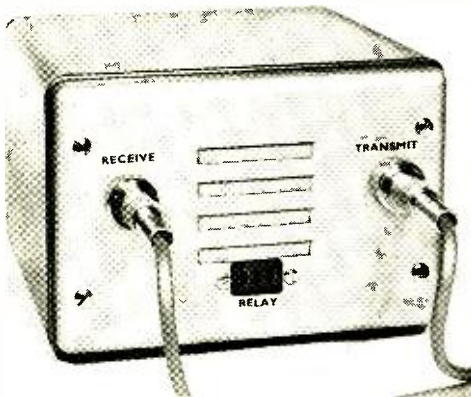
Fig. 4. By locating the receiver and transmitter output and input connectors on the rear cover, the entire package takes on a clean professional look.
