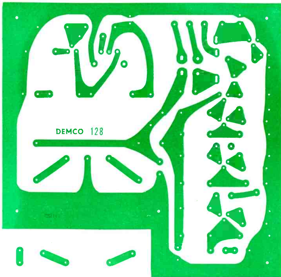
Fig. 2. Actual size photo of conductor side of printed circuit board. Components can be mounted on any type of chassis, but care should be exercised to prevent stray leakage, or coupling.
