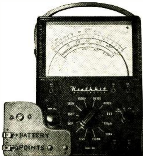
All parts, including banana plugs, are mounted on a piece of fiberboard shaped to conform to the meter.
