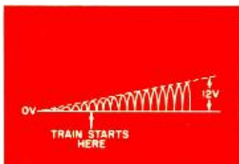
Fig. 1. The ordinary power pack is nothing more than a full-wave rectifier whose output is a pulsating d.c. voltage with peaks that look like the waveform above. For most locos, the average power required for starting is much too high for a smooth start, and the trains pull out with a sudden jerk, and at a speed not akin to real railroading.
