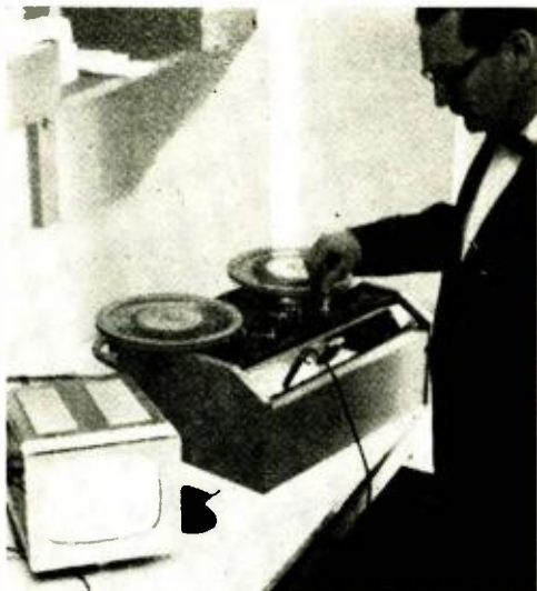
Wesgrove is one of the two British manufacturers that introduced low-cost TV tape recorders. This particular machine is available as a kit for $400.
