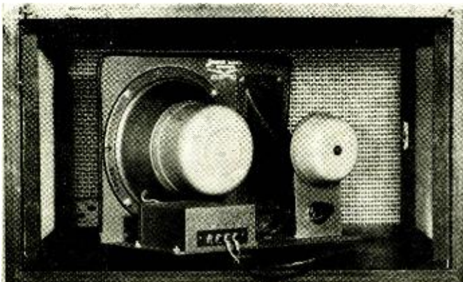
Almost every speaker has some directional characteristics, but Jensen's SS-100 was a bona-fide attempt to use "direction" to solve the stereo listening area problem. In the SS-100, the mid-range and treble speaker were mounted on a platform and could be aimed at the audience.
