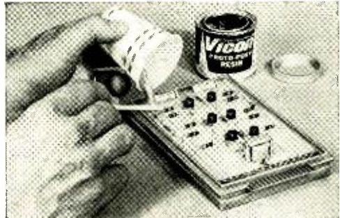
Fig. 15. This "Proto-Board" circuit can be fitted with a frame as shown and covered with a special epoxy resin compound.
