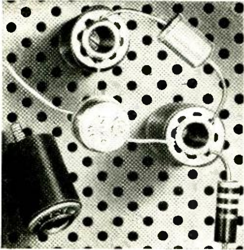
Fig. 7. Component leads are pressed into holes in top of ETA "Flexi-Klip" connectors.
