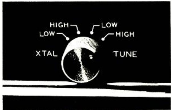
Some of the police/fire receivers offer a crystal-controlled tuning position. You can obtain specially ground crystals for use on specific channels.
