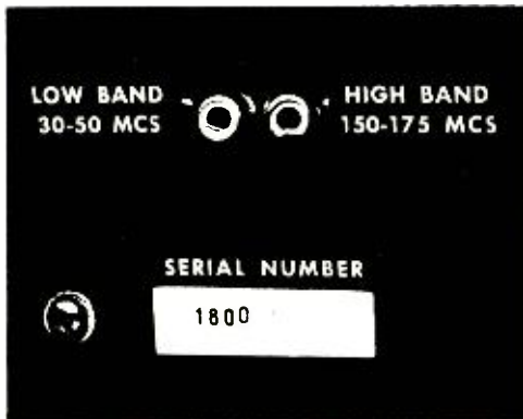
Two-band receivers work best with separate antennas for the high and low bands. In this Utica receiver, the antenna jacks are of the RCA phono type.
