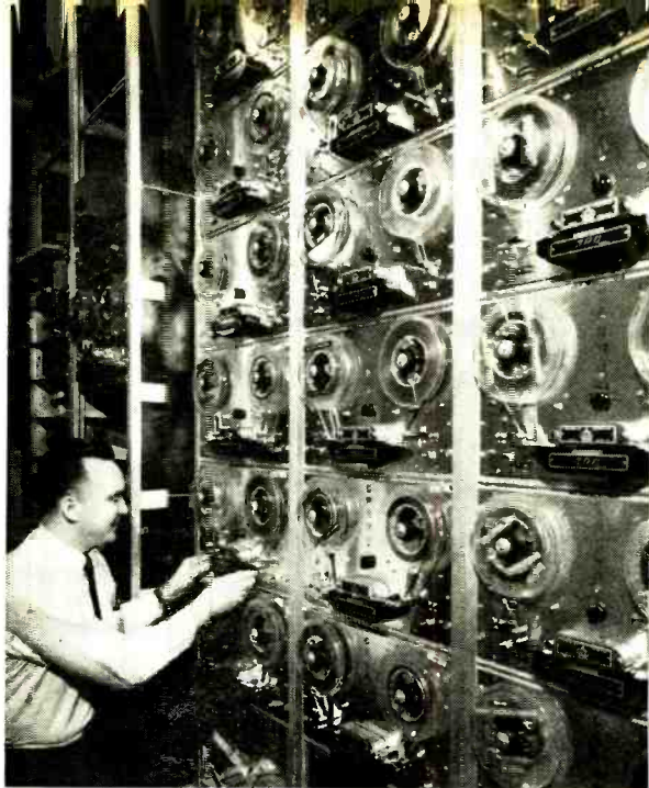
Behind the scenes at the Bell System exhibit is the tape deck which provides sound for the displays. The 30 tapes give visitors stories ranging from how the laser works to a history of communications.
