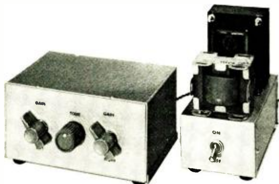
Amplifier's low silhouette and finished appearance is achieved by mounting tubes on the rear apron.
