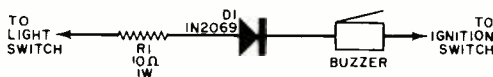
Light Minder uses three components; R1 is omitted in 6-volt cars, leads reversed for positive ground.
