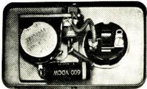
The heat sink on the inside of the case and the dial plate on the outside are held in place by a rivet (hidden by the capacitor) and the potentiometer nut.
