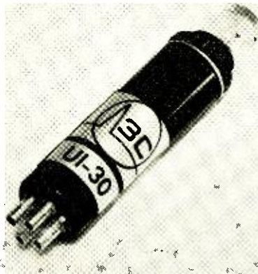
Fig. 2. Plug-in lamp indicator package contains a high-voltage transistor driver which can be triggered by a low voltage from a transistor circuit.
