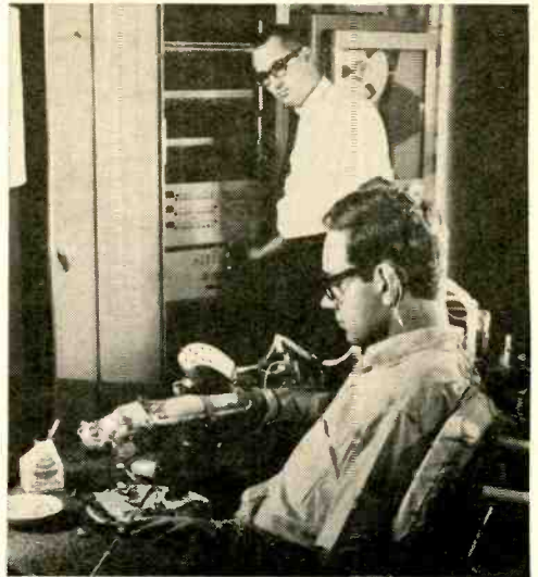
Computer (background) holds programs for arm-aid activities such as eating, shaving, and drinking.
