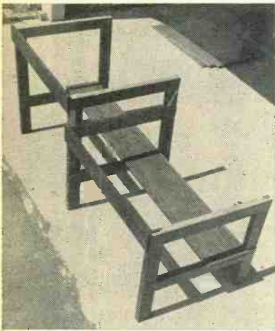
The work/op bench in various stages of assembly. Use screws and shun glue, and you can easily take it apart for moving, set it up later on.
