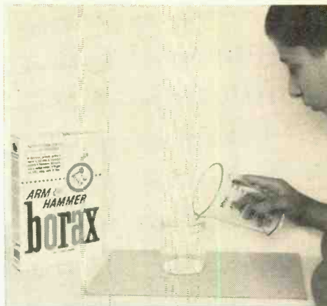
The first step in making a chemical rectifier is to dissolve Borax in water—peanut butter jar is used.
