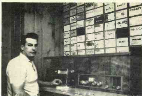
Larry Fritz, W8LHY, of Cleveland, Ohio, dressed up his station by building a single cabinet to house both his transmitter and receiver. The transmitter (on the right) is also home-constructed, and has worked 44 states and Canada in about three months.
