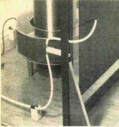
Leads are soldered directly to capacitor plates. Note use of stand-off insulators.
