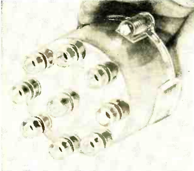
Some distributor caps will not withstand the extra high voltages generated by the high turns-ratio coils. This transparent distributor cap was designed for ignition systems where voltage leakage is a problem. Called the "Transpark," it is sold by Estes Engineering Co., 1639 W. 135 St., Gardena, Calif., for only $6.95.
