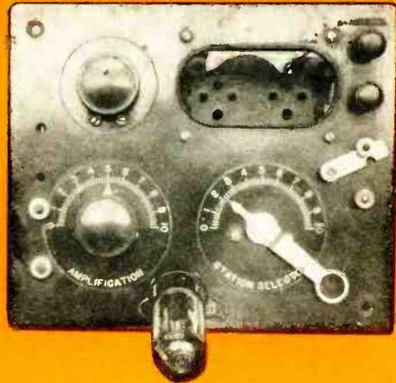
The first one-tube battery receivers used the WD11, a 1½-volt triode. This is RCA's Radiola which came shortly after Westinghouse's Aeriola receiver.
