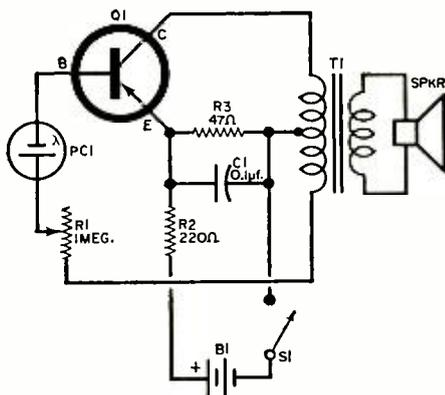
cillation. Transistor  $Q1$ 's base bias is furnished through  $R1$  and photocell  $PC1$ ; thus, the transistor's operation depends on the amount of light striking the photocell. Series current-limiting resistor  $R2$  and shunt resistor  $R3$ , bypassed by  $C1$ , provide proper operating voltages. Power is supplied by a 9-volt battery,  $B1$ , controlled by a s.p.s.t. switch,  $S1$ .
