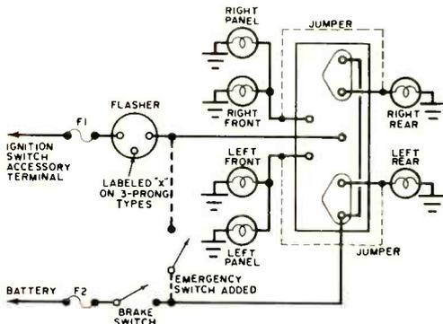
on when the brake pedal is pressed—an additional safety measure and one that is required by some new state laws. When the emergency switch is closed, all four front and back lights flash. In most cars, the jumpers simply tie together the two sets of wires at the distribution panel.
