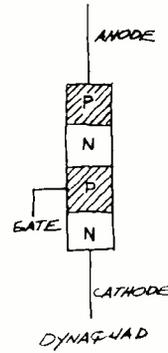
It is possible, of course, to provide an electrical connection for the second as well as the first, third and fourth layers in a four-layer device. In this case, we have another gate electrode and, to differentiate between the two gate connections, the one nearest the anode is called the *anode gate* ( $G_A$ ), while the one nearest the cathode is termed the *cathode gate* ( $G_C$ ).
