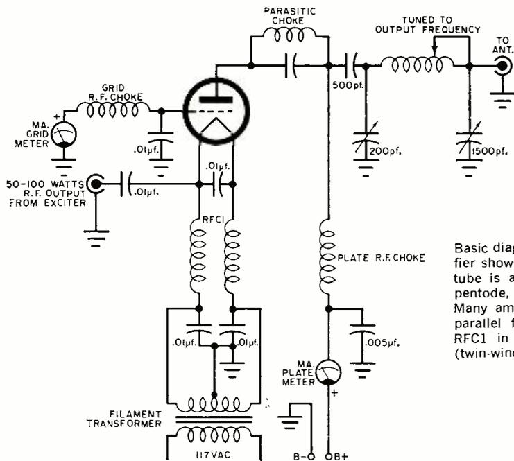
Basic diagram of grounded-grid amplifier shows its inherent simplicity. The tube is a high- $\mu$  triode, tetrode or pentode, with all grids grounded. Many amplifiers use several tubes in parallel for increased power. Choke RFC1 in the heater line is a bifilar (twin-winding) high-current r.f. unit.
