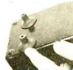
You can make some dandy rubber feet for your instruments from simple suction cups. Rubber cement will hold them in place, or, if you like, a small hole can be drilled in each suction cup and a bolt used to attach it to the cabinet. The suction cups are resilient, and provide good shock protection.
