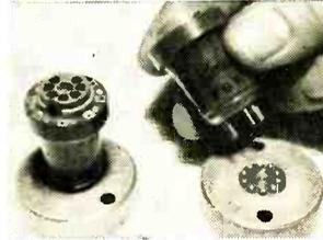
To keep your adapter sockets handy and safe, there's no better place to put them than in your tube pin straighteners. The adapter socket pins will be protected, and the sockets themselves will be ready for use at all times.
