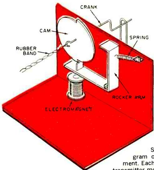
Simplified diagram of an escapement. Each pulse from a transmitter moves the cam.
