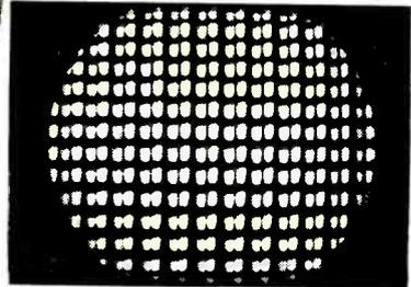
The secret of color TV is the convergence or joining up of the three electron beams so they hit the proper miniscule green, red, and blue dots on the TV tube face. Above right, the beams are badly out of convergence. They must be properly converged by manipulating controls at right. Proper convergence and linearity is shown (the dots are white) below.
