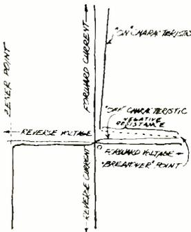
by a gate signal . . . afterwards, it can be returned to its stable "off" state only by dropping the anode-cathode voltage to a low value. Slightly modified forms which can also be switched off by the application of a reverse bias to the gate are called *Trigistors* (Clevite-Shockley) and *Transwitches* (Transitron). A germanium version of the device is called a *Dynaquad* by its manufacturer (Tung-Sol).
