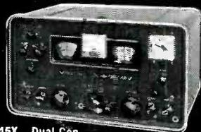
**HQ-145X** — Dual Conversion general coverage SWL and Ham receiver with single crystal control channel. **\$279.00**
