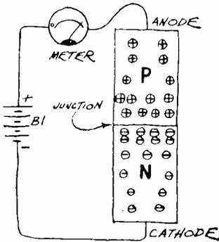
Diodes are essentially a junction of *p*- and *n*-type semiconductor materials. The diode derives most of its capabilities from its nonlinear, unidirectional electrical characteristics, i.e., its ability to conduct freely in one direction while acting as a high resistance or open circuit in the opposite direction.
