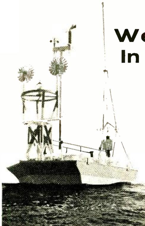
Special anchor line, made largely of buoyant nylon, holds MAMOS secure in up to 18,000 feet of water.
