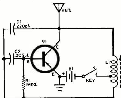
battery voltage is not critical and  $B1$  can supply from 3 to 9 volts; the power supply, therefore, may be either a small 9-volt transistor battery or may be made up of several series-connected flashlight cells.
