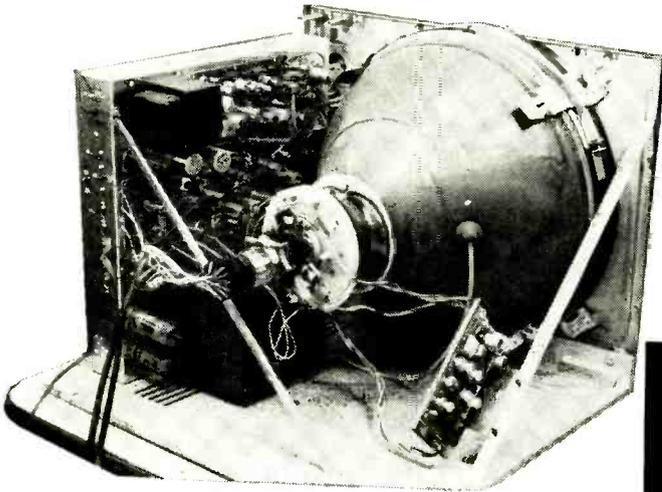
For custom mounting, the GR-53A looks like this. A console cabinet is available from the manufacturer for \$49 extra. Picture tube is held in place by metal bands attached to the mask. Chassis is upright, with power supply cage in the box at the lower left corner.
