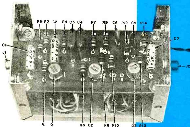
Refer to the schematic diagram on the facing page to locate the components in photo above.
