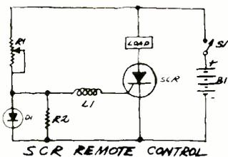
Commercial SCR's are sold in sizes with current ratings of less than 1 ampere to well over a hundred amperes, and with voltage ratings up to 500 volts or more. While standard SCR's can be turned "on" by the application of a trigger signal to their gate—and "off" only by dropping or reversing the anode-cathode voltage, there are several new types which can be turned "off" by the application of a reverse bias trigger to their gate.
