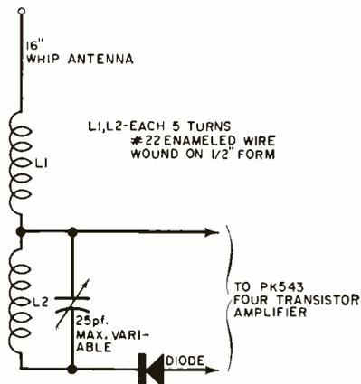
listen to the airport control tower from my house using a 16" whip antenna. The circuit is inexpensive, and gives good loudspeaker volume from any point around the airport.
