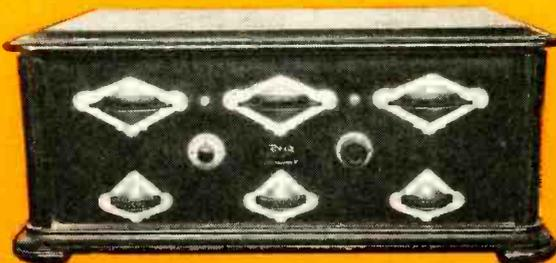
If you were under the impression that radio kits are a modern innovation, here's proof to the contrary. The 1924 Freshman Masterpiece kit above, a five-tube TRF model, was the pride and joy of the electronics hobbyist of that era. All three dials had to be adjusted to tune in a broadcast station.
