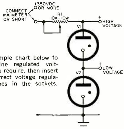
Use simple chart below to determine regulated voltage you require, then insert the correct voltage regulator tubes in the sockets.
