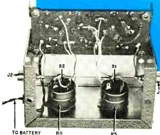
tive filter. Potentiometer *R11* is used to vary the cutoff frequency of the filter from approximately 3000 to 6000 cycles. In the "out" position of *R11*, the normally closed pole of switch *S2* opens and breaks the signal connection to *R11*, while the normally open pole of the switch closes and shunts the signal around the filter.
