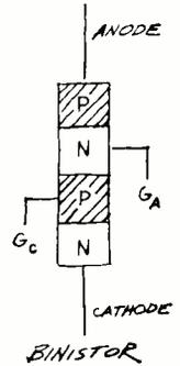
One manufacturer of the four-layer, four-connection "diode" suggests that the anode gate connection be used as an output terminal. The device is then called a *binistor*, and new designations are assigned to each of the electrodes. The anode is called an *injector*, the anode gate a *collector*, the cathode gate a *base*, and the cathode the *emitter*.
