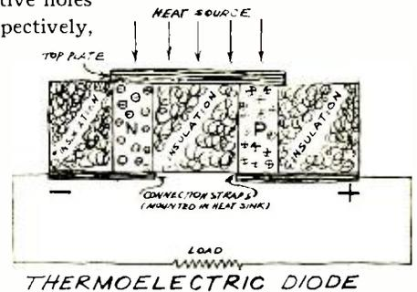
undergo thermal diffusion from the high- to the low-temperature side, developing a potential difference. This voltage can be used as an effective power source for a standard electrical load as long as a temperature difference is maintained between the two sides of the device. Thus, the unit becomes a heat-to-electrical energy converter.
