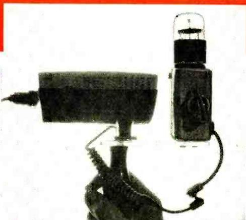
All it takes is a triggering flash to set the slave strobe off. Adjust potentiometer R2 for best sensitivity.
