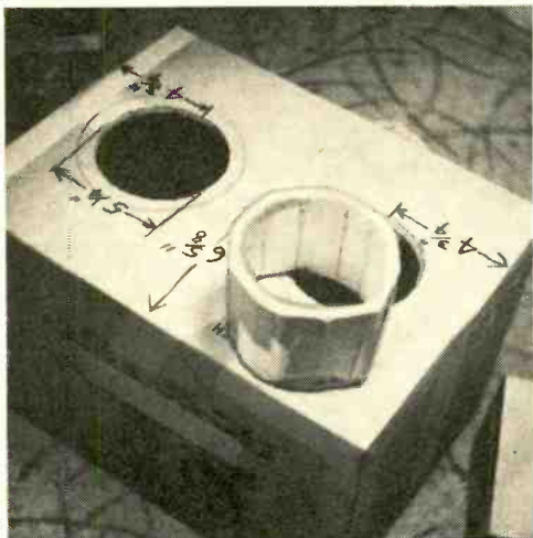
The duct is made by rolling a strip of 3\frac{1}{4} " x 35" cardboard into a 5\frac{1}{4} " i.d. tube; fasten with tape.
