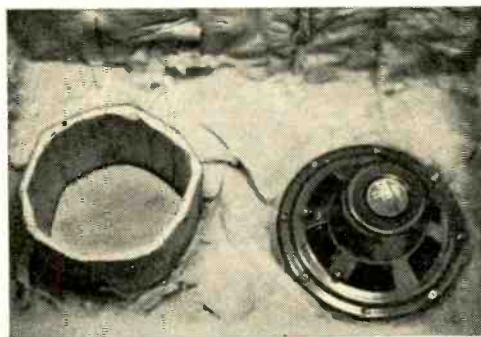
The speaker is bolted to the reinforced cardboard bottom—punch holes for the screws with ice pick.
