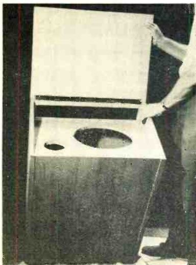
Enclosure with speaker board in position.
