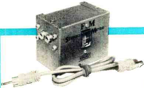
Simple diode MPX Meter—no transistors, batteries, switches—will work with many tuners having high-output ratio detectors.
