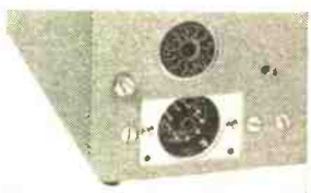
ACCESSORY SOCKET on rear panel (above power cord receptacle) for instant attachment of "Tone Alert".
