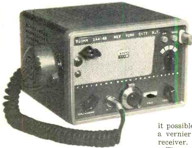
This is the author's version of a "Double-Duty" EICO Model 772. The nameplate shows his original CB call—2A4148. New control functions are indicated in the photo on the facing page.
