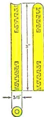
Fig. 3. Grounding stub post is made of brass or aluminum rod. Both ends are drilled and tapped to 1" to accept 10-32 screw.
