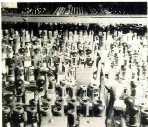
Acres of tubes? Almost. Many are 12AU7's connected in "yes-no" type, flip-flop computer circuits.
