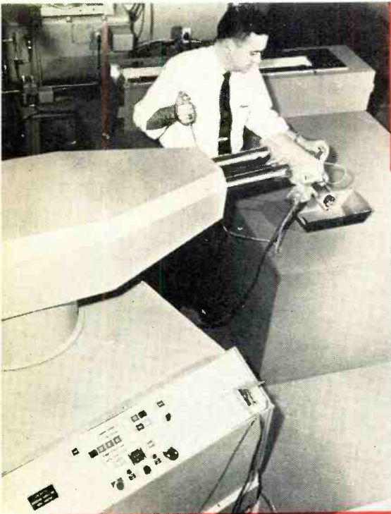
STUDENT ROBOT is "Unimate," which has a brain and can memorize 200 separate steps after being led through them by hand; "teaching" process is shown.
