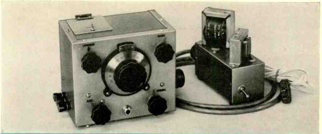
All-wave receiver and its power supply, ready for use. Since power requirements are comfortably low (about 150 volts d.c. @ 25 ma., and 6.3 volts a.c. @ 1.0 ampere), you may be able to "steal" the power from an existing receiver or amplifier and thus save yourself the trouble of building a separate supply.
