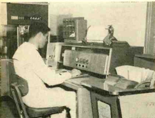
Operator at console of RAMAC electronic computer instructs machine to locate and type out information previously stored on magnetic "memory" tracks.
