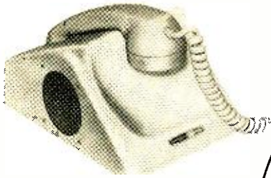
Fig. 2. Block diagram of typical telephone amplifier. As in GD-71 Heathkit (photo above), basic elements include inductive pickup coil, transistorized amplifier, and speaker.
