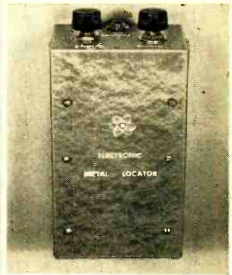
Completed Lodestar fits snugly in a 5¼" x 3" x 2½" box. To operate it, simply plug the sensing coil into jack J1, headphones or speaker into jack J2.
