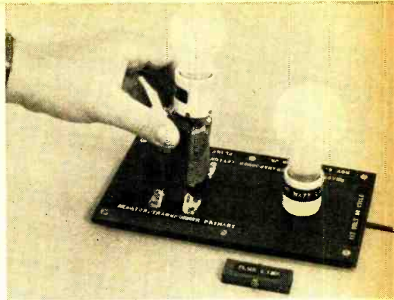
Fig. 3. Here transformer action is demonstrated by placing L2/I2 atop L1 . Enough voltage is then induced in L2 to make 15-watt lamp I2 glow brightly.
