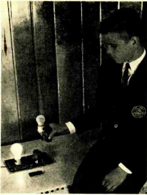
Fig. 1. Operator removes flux link from choke L1 , reducing inductance of the choke and causing series-connected, 60-watt lamp L1 to glow brightly.
