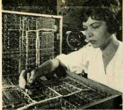
The equivalent of a private telephone system, the Martin Co's RACEP (left) needs no wires or central switching facilities. Another new communications device, Hughes' vocoder (above), "condenses" speech into basic sounds, reproduces it artificially.
