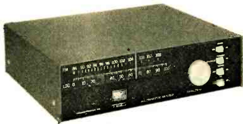
Fig 1. Transis-Tronics' Model FM-15MX FM stereo tuner draws astoundingly little power from the a.c. line, thanks to its completely transistorized circuitry. A perfect match for the company's Model S-15 all-transistor stereo amplifier, the FM-15MX uses 20 transistors and 9 diodes, and features its own built-in regulated power supply.
