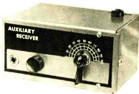
Completed receiver (above) needs only an earphone, an antenna, and a battery to operate. Note that the entire receiver is housed in front portion of the case (below).
