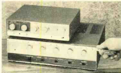
Fig. 7. These two Knight stereo amplifiers have about the same power rating, but the all-transistor unit (on top) is dwarfed by the vacuum-tube version.
