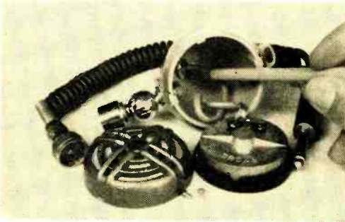
Astatic's Model 151 ceramic mike can be disassembled and a new cord soldered directly to the cartridge.
