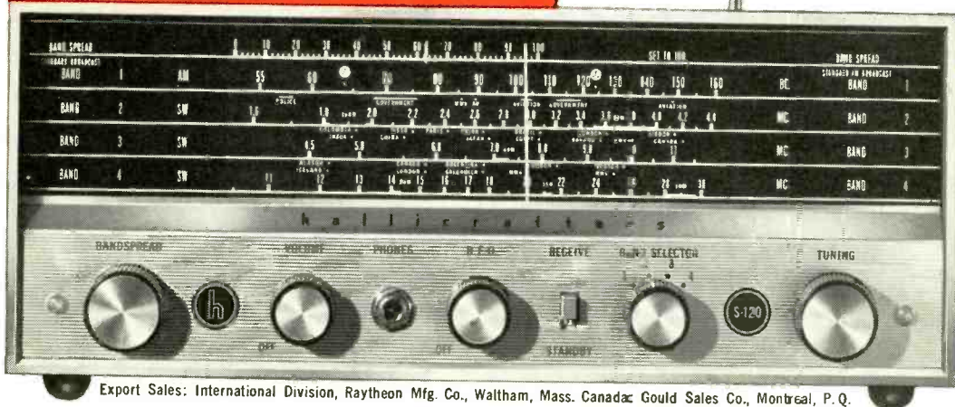
SX-110 Receiver—$189.85. Standard broadcast. Three short wave bands (1550 kc-34 Mc.). Slide rule electrical bandspread dial. Built-in "S" meter, antenna trimmer, crystal filter. Uses R-48 speaker ($19.95).
