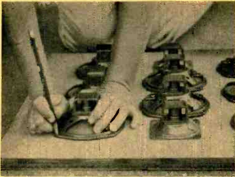
Begin construction by placing speakers on speaker boards and marking through each mounting hole with a soft pencil.
