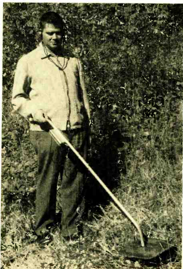
Fig. 1. The Model 100T metal locator, produced by Electronic Applications Co., employs two oscillators and a detector/amplifier. Metals alter inductance of pickup coil (see photo), changing frequency of Q1's oscillations and tone heard in headphones.
