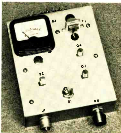
Placement of parts on modulator chassis is shown in photos above and at right. Author used relatively large chassis to have plenty of room for wiring.
