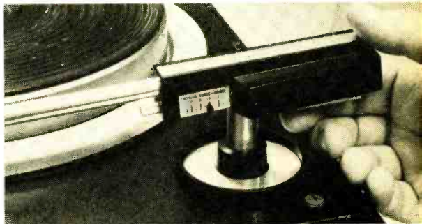
The M232 arm is statically balanced by a counterweight which is adjusted by knurled knob under arm. Tension is set by spring adjustment to 3 grams.
