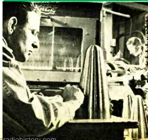
Technician checks thickness of Explorer satellite nose cone with ultrasonic gauge. The sharp vertical line on the scope face indicates thickness to within one one-thousandth of an inch.
