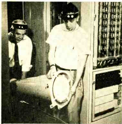
Cathode-ray tube in electronic central's "flying spot store" (below, left) is a photographic "memory" device capable of storing over two million "bits" of information. Tube sweeps spots on film (left)—over 30,000 to each 1½" square—which are either clear or opaque and which pass or withhold the beam of light accordingly.
