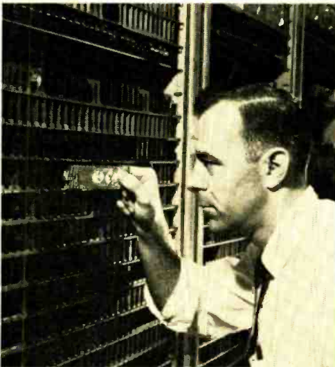
Control center (three photos, left) of world's first all-electronic telephone central office, now serving customers in Morris, Ill., is but a portion of overall network shown in block form below. The system was developed by Bell Telephone Laboratories.
