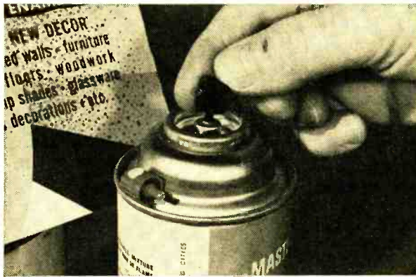
4 An accessory spray head (below) produces a "spatter-type" finish for old cabinets, enclosures, panels.
