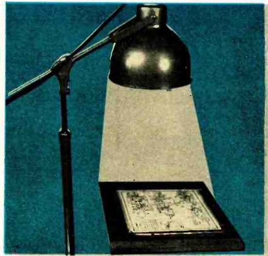
Sun lamp provides illumination in this set-up. Drawing lies on top of sensitized paper.
